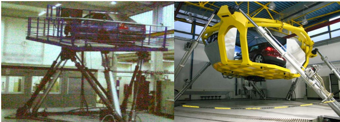
Fig. 1-5: Left – a full car simulator situated on robust hexapod platform in BMW Right – one of the European latest simulators by Simtec and DLR, Bruunschweig
