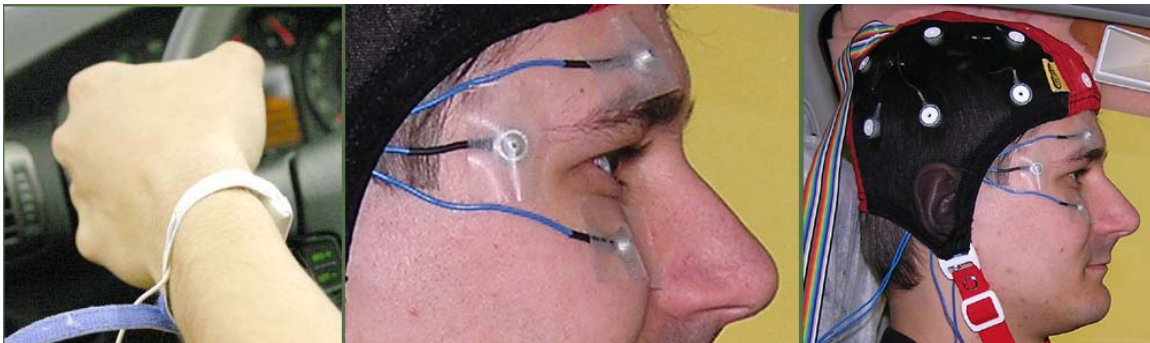
Fig. 7-14: The tested driver equipped with heart beat recording, EOG electrodes and the EEG cap
