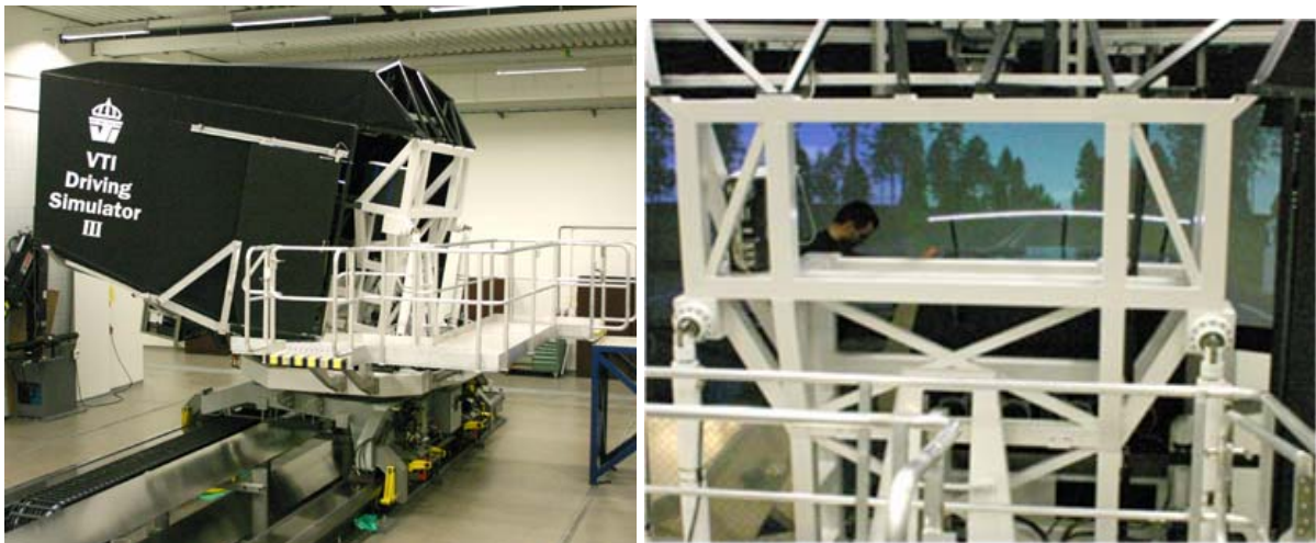
Fig. 1-4: A hybrid motion platform for simulator VTI in Linkeping (Right - an inner view)
