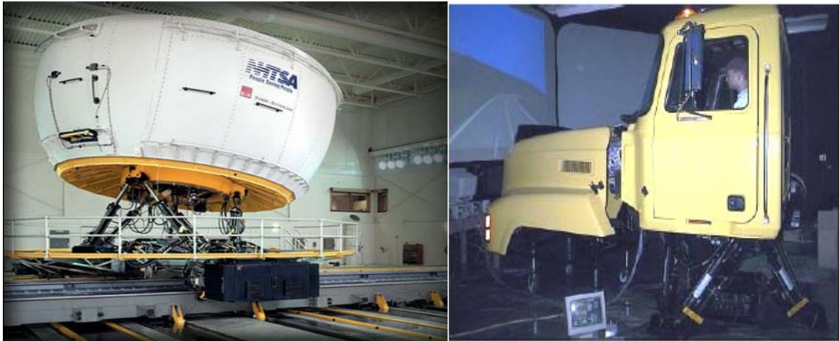
Fig. 1- 3: Left - Perhaps the most advanced motion based simulation system NADS Right- The still based Pennsylvania Truck Driving Simulator
