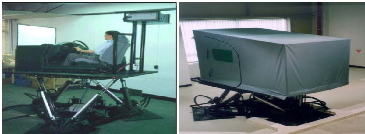
Fig. 1-2: Hexapod based simulator of Kookmin University in Seoul
