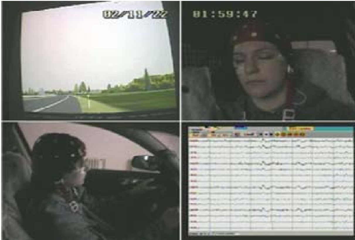
Fig. 7-10: The standard form of our driver's video record completed with EEG record (right bottom) in time of driver's micro-sleep
