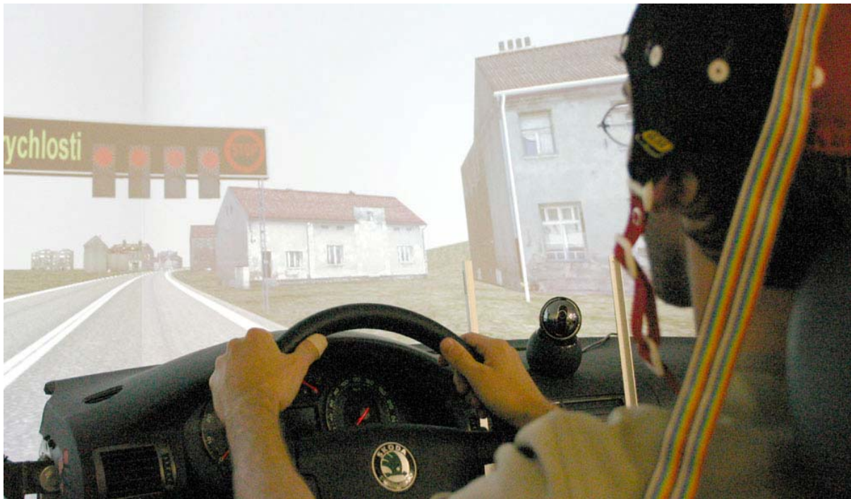
Fig. 7-7: The tested driver equipped with EEG cap and heart beat recording sensors (the Compact simulator type I – a), Light simulator type I version 2005– b)).
